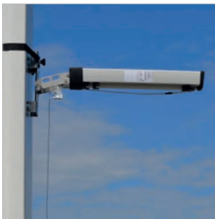
The tool can be easily mounted to any panel antenna by using different adapter plates, a special mounting belt or the universal mounting support.
